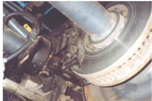
Fig. 5. View of a brake disc made of an aluminum-ceramic alloy by Knorr-Bremse
